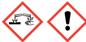
Corrosion Exclamation mark
