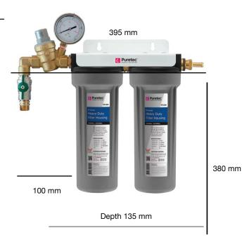
The CD501-CCA is a twin-stage filter system with a 5 micron sediment removal cartridge and a 5 micron granular activated carbon cartridge.
