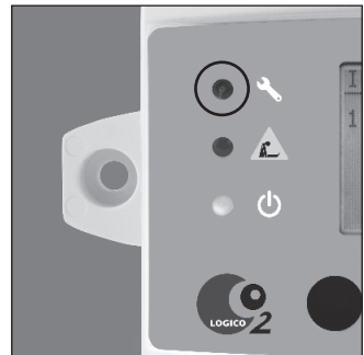
System fault indicator
