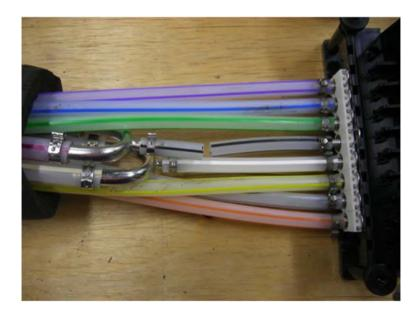
3. Attach approximately 220mm of black soda supply tubing to a 6mm elbow. Attach elbow to the 6mm supply barb of the soda "U" bend.
