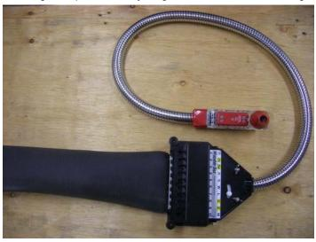
Remove approximately 200 to 250 mm of python insulation from where the python connects to the bar gun manifold.
