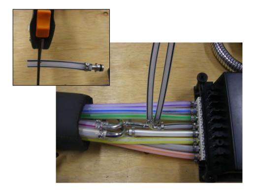
5. Select the Mother syrup line that the volumetric valve is to be connected too. (The purple No2 – Dry Ginger line has been selected as the example in this instruction sheet). Cut purple No2 syrup supply tube approximately 80 mm from the manifold.
