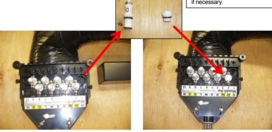
14. Replace the DR Button with the "M" button supplied. (The DR Button has been selected to be replaced as the example in this instruction sheet).
