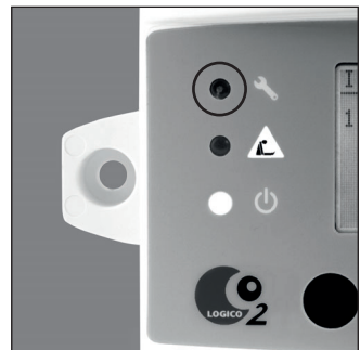
System fault indicator
